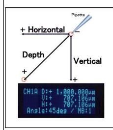
The digital scale in the drive unit calculates the position in real time.
