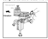
However, still it is extremely difficult to control a pipette in a precise way only with a manually operated manipulator in high magnification. Therefore, when an experiment requires higher total magnification of more than 100 times, remotely controlled micromanipulators are commonly used.
