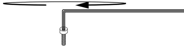
It is important that the tip of the wrench is inserted up to the bottom of the recess of the screw head. It follows that when the wrench engages with the recess exactly, the rotation axis becomes stable. As the contact area is at maximum, make sure that the torque does not go in the wrong direction, damaging the edges. Twisted and wrenches with damaged tips can cause tension which is dangerous. These types of wrenches should not be used.
