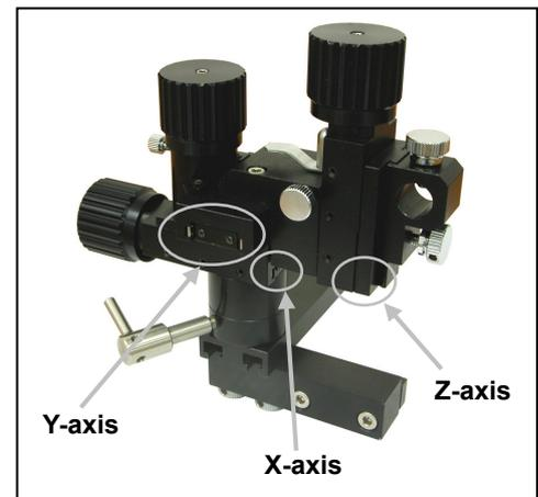
The ideal setting for all axes of a coarse or fine manipulator are set at the center of the working range, while a pipette tip positions at the center of the optical axis of the microscope.
