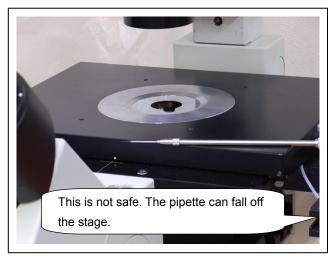
If the injection holder is simply put on the microscope stage, it can fall off the stage if the injector tubing is accidentally pulled. The injection holder can also lean downward and leak injector oil. In such cases, HIK-3 / HIK-4 Pipette Holder Keeper can be useful.
