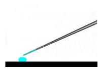
By using a microinjector together with micromanipulators, you can make a tiny drop of adhesive agent or a marker in a desired location.
