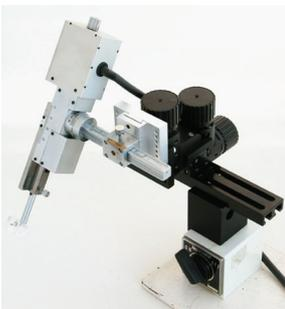
The DMA-1511 was originally designed to be used in combination with SM-11 stereotaxic micromanipulator. However, in response to a customer’s request for utilizing the DMA-1511 as a single-axis digital micromanipulator, Narishige customized adapting parts to connect a three-axis coarse manipulator and a magnetic base so as to allow for flexible installation.
