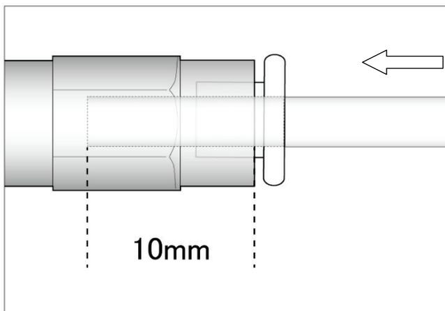
When reconnecting, insert the tubing by 10mm (all the way) into the tube fitting. If the tubing is not inserted deep enough, it can cause air leakage that deteriorates pressure control ability of the injector and makes the injector uncontrollable.
