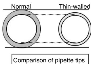
The inner diameter of the normal glass capillary is 60% of the outer diameter, while it is 80% in the thin-walled capillaries. When the inner diameter is equal in the two types of the pipettes, the thin-walled type has a smaller outer diameter than the normal type has. This helps diminish damage to cells. On the other hand, the thin-wall type is more difficult to process into a pipette because it is not as strong as the normal type.
