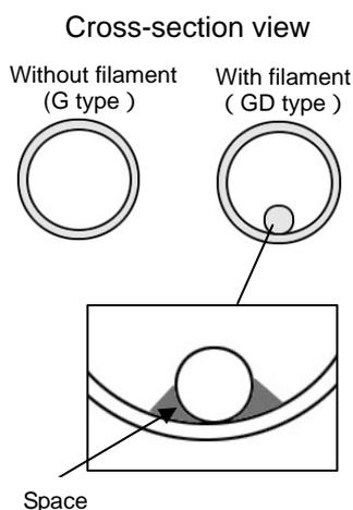
One of the biggest differences in glass capillaries is whether or not it has a filament in the tubing.
