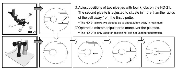
%The HD-21 is also mounted on manual manipulators such as the M-152. Mounting bar on the HD-21 is 8mm in diameter.
